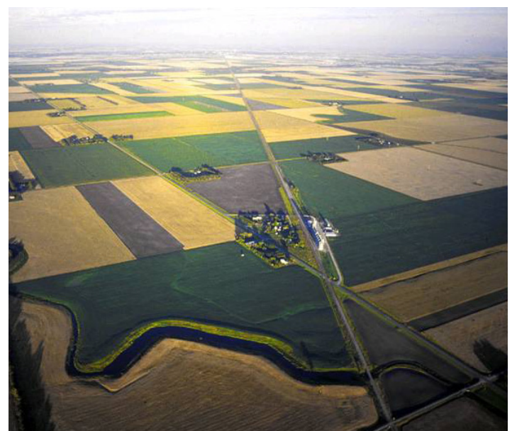
Figure 4 | Evidence of the Public Land Survey System. Visible evidence of the Public Land Survey System (PLSS) across the United States can be seen above in the aerial landscape photos by Alex MacLean. Above image: “Railroads Across Survey Landscape: Castleton, South Dakota.” 5
